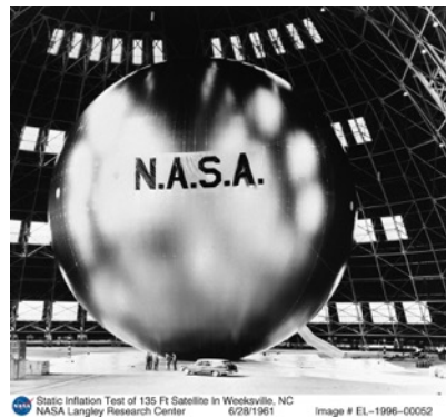
Static Inflation Test of 135 Ft Satellite in Woomville, NC NASA Langley Research Center 6/28/1961 Image # EL-1996-00052
